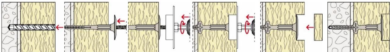
1. Drill hole by corresponding drilling method
