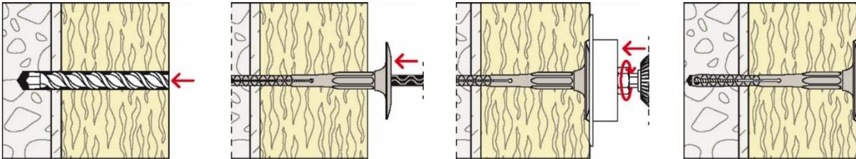
1. Drill hole by corresponding drilling method
