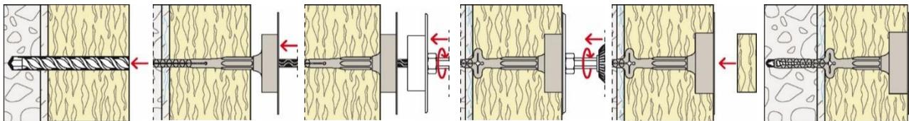
1. Drill hole by corresponding drilling method
