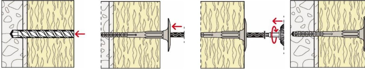
1. Drill hole by corresponding drilling method
